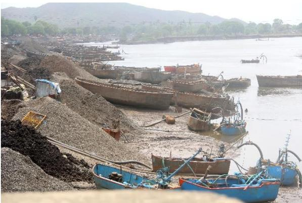
Figure 5 : Sable extraction - Sand mining with suction pumps
