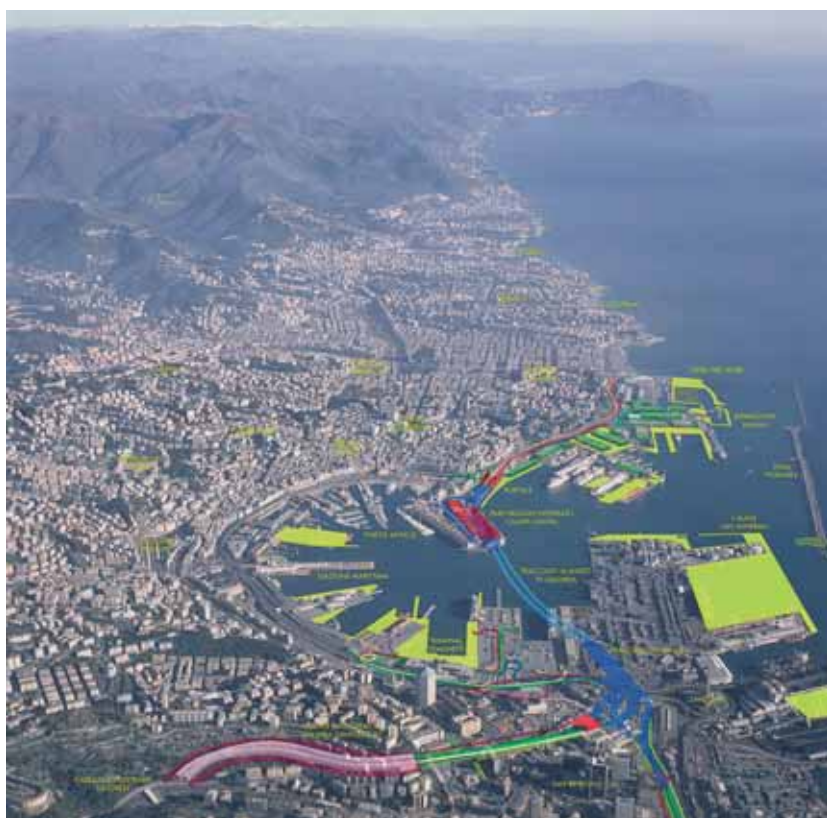
The areas for port development (in yellow) and the project to dig a road tunnel under the port (in blue) which would open up the possibility of doing away with la Sopraelevata, the road viaduct which cuts the city off from the port.
