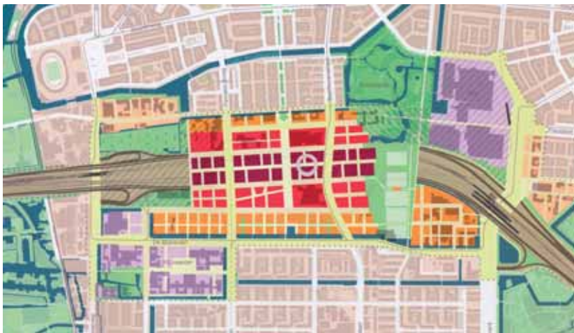
The Masterplan Zuidas, approved in 2004, showing the continuity of public space on both sides of the underground infrastructure.
